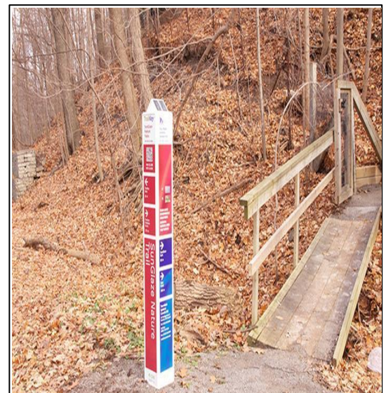
A photo of trail identification signage that incorporates large-print, tactile and audible information.
